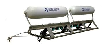
**The Delta Sparker** is the most powerful sparker available in the Applied Acoustics' range and is intended for deeper penetration sub-bottom profiling.
